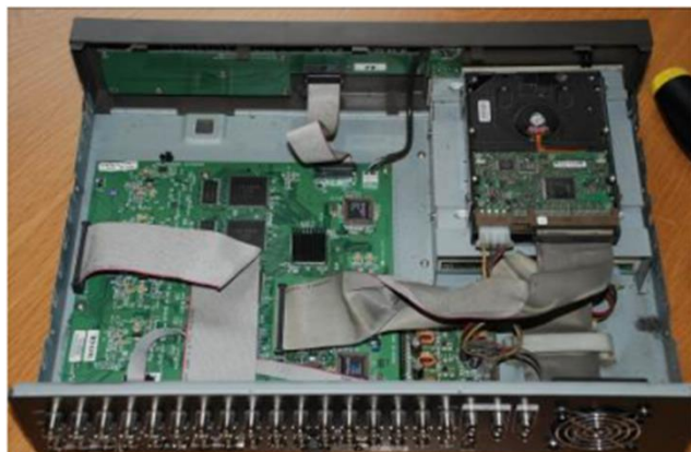
Fig27. Internal view of a DVR
