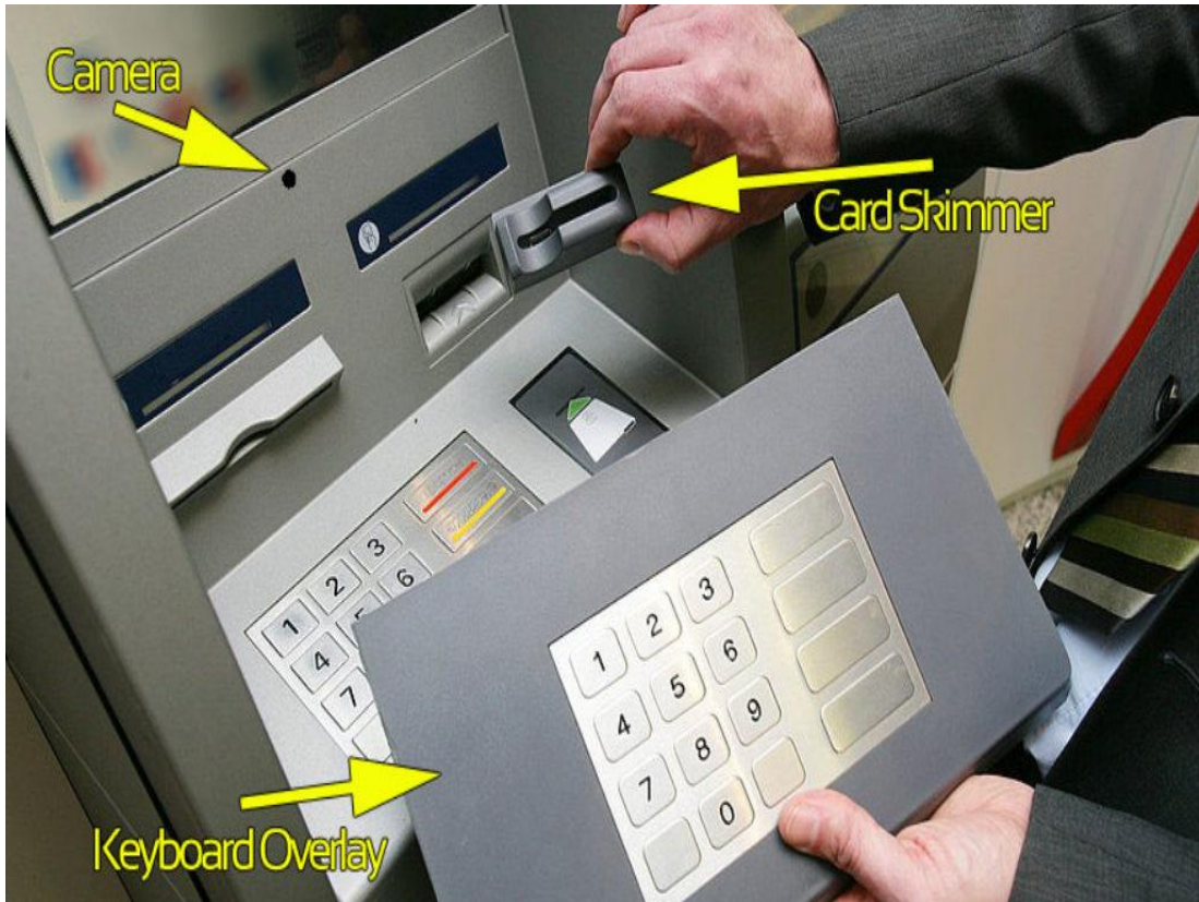
Fig 21. Camera, Card Skimmer and Keyboard Overlay
